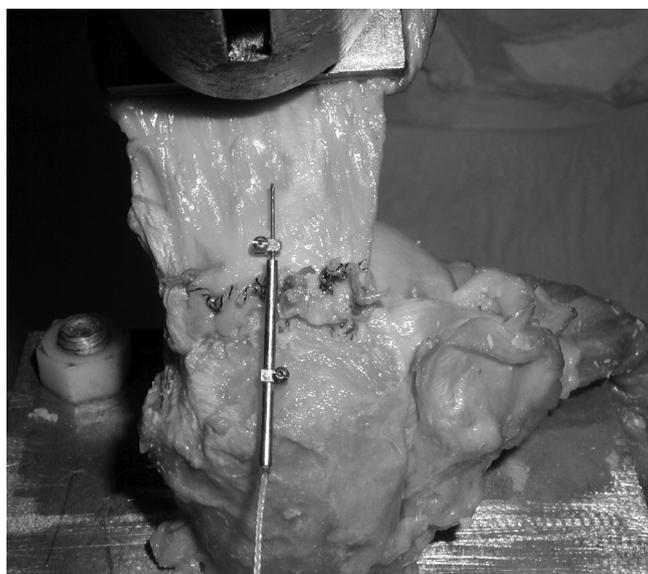
Figure 5. Strain gauge applied for testing displacement.
